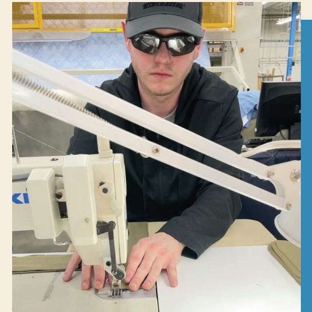
Timothy Jones uses an adapted single-needle machine for making collars
